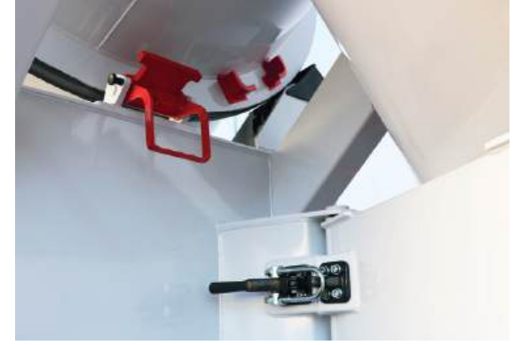
Kazan Emniyet Kiliti ve Kilit Sistemli Tek Oluk Kolu Drum Hydraulic Lock and Single Chute Arm with Brake
